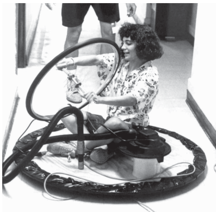
Fig. 6. Kathryn Cole and her hovercraft formed a nearly isolated system that reacted to the inversion of a spinning bicycle-wheel gyroscope. 6
