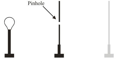
5. From **one point** on the bulb, draw two rays that go through the pinhole (one at the top of the hole, the other at the bottom). Explain in words how increasing the size of the pinhole affects the brightness and sharpness of the bulb reproduction on the screen.
