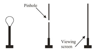
2. Now draw **two rays** (one from top of the bulb, the other from the bottom of the bulb) that travel through the pinhole and reach the screen. Draw several eyes that would be able to see the light that reaches the screen. Explain in words how an inverted reproduction of the bulb is formed on the screen.
