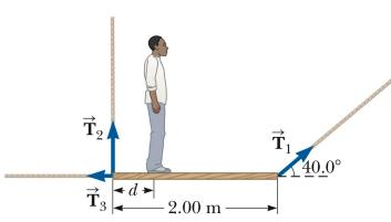
The uniform plank weighs 200 N and is supported by three ropes as shown. A person weighing 750 N stands a distance d = 0.3 m from the left end of the plank.
