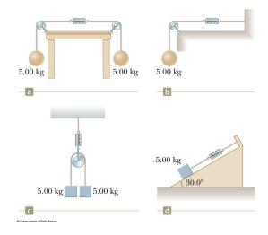
The spring scale gives the tension in the string just as if the scale were replaced with a length of string. In case a, the scale reads the weight of a 5 kg mass, just as if one end of the scale were attached to a wall as in case b. The scale in case c shows the weight of 10 kg. The scale in case d shows only  $mg\sin\theta$ , which is half the weight of a 5 kg mass.
